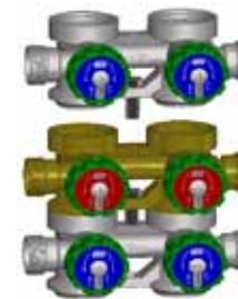
Insert the screw art.8551 in the hole placed between the two connections, as indicated in the figure. Before assembling the manifold, make sure that the sealing O-Rings (art.8350 2824) have been mounted.
