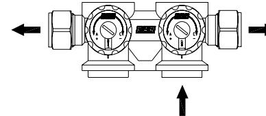
Each stop valve is provided with a silk-screen printed disc, that permits the exact identification of the terminal connected to each outlet during replacement or maintenance of a fixture.
