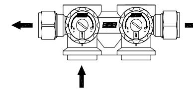
**RIGHT (CHROME-PLATED):** This is the manifold that permits to connect pipelines with flow entering from the right. On the manifold itself an arrow indicates flow direction.
