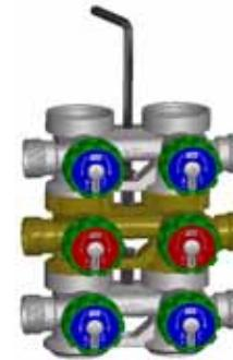
To assemble a manifold to another one, insert the Allen wrench art.6251 in the upper hole, in this way you can handle the wrench with easiness. Then tighten strongly.
